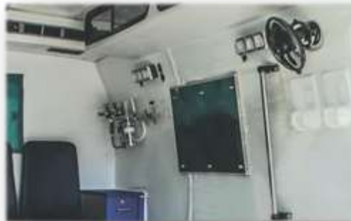
Reinforced Side wall to mount Medical Equipment's
