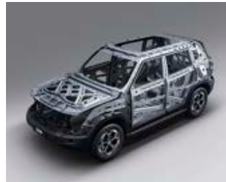
SAFE BODY STRUCTURE 85% HIGH-STRENGTH STEEL
